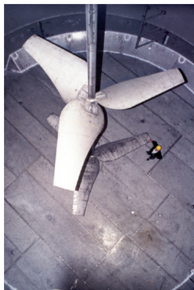
Vertical agitator for paper chemicals. Double-acting propeller for viscous liquids and pulp applications.
